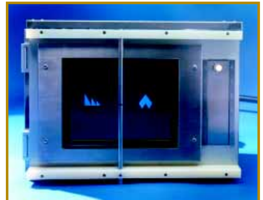
Picture shows the set-up for marmosets with a licker placed across the screen. (Alternatively a remote licker can be attached.)
